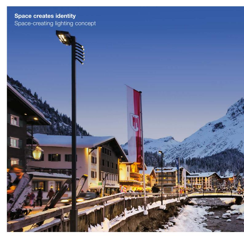
The mountain river defines the townscape during the day – and now the same can be said at night thanks to the new lighting system. LED tubes attached to the lighting columns direct light towards the riverbank and the surfaces of the adjoining walls.
